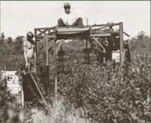
Designed by Tom Darlington, this mechanized blueberry picker is one of the many local blueberry industry innovations.
